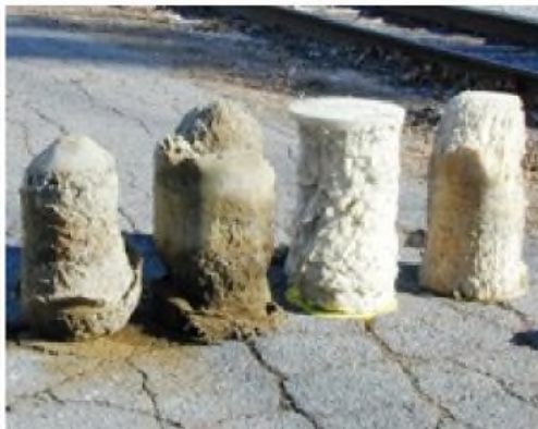
Pigs run through a scaled 8" water line. Left Two Pigs: RBS, medium hardness. Right Two Pigs: YBS, soft type
