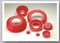
Girard Scraper Cups and Conical Cups range in size from 2" to 56". Both are available in most of these sizes. Girard Polyurethane cups and discs are designed for maximum abrasion resistance, elongation, shear strength and chemical resistance. This assures peak performance under the largest variety of pipeline conditions.
