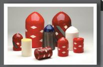
Girard Polly-Pigs, constructed of open cell polyurethane foam, are available in light, medium and heavy densities. They are designed to negotiate pipeline configurations that other pigs cannot, such as "tees," elbows and multiple diameter changes. With over 28 different models to choose from, Polly-Pigs can do everything from light cleaning and drying to removal of heavy scale.
