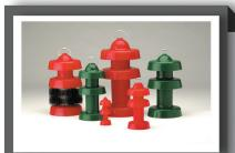
The Girard Turbo-Magnum<sup>™</sup> is a one piece, all polyurethane pig available with either 3 or 4 cups. The hollow center allows for maximum flexibility while negotiating tight radius bends and other pipeline features.
